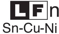
Indicates lead-free solder of tin, copper and nickel
