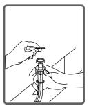
**CAUTION:** Filters of water inlet valves may be clogged due to contaminated water faucet or lack of necessary maintenance or valves may be broken down, causing water leaking into your machine continuously.
