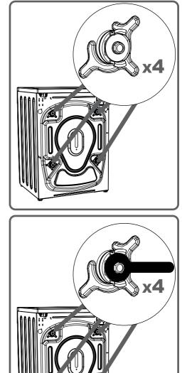
For this reason, transportation safety screws shall be loosened by being rotated in counter-clockwise using an appropriate wrench.
