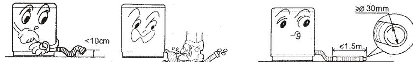
3. Cut the drain hose if it is too long. Cut the front end of the drain hose slantingly to make drainage smoothly.
