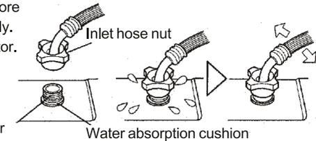
**Cautions:** When install the washing machine, please use the new hose assy along with the washing machine, old hose assy can not reuse.
