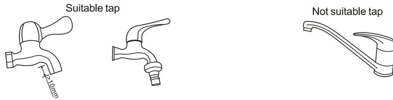
The front end should be longer than 10mm. The tap exit end face should be flat and smooth, if not file it to avoid leakage.
