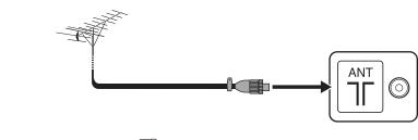
If your outdoor antenna uses a 75-ohm coaxial cable with a standard DIN45325 plug (IEC 169-2), plug it into the antenna jack at the rear of the set.
