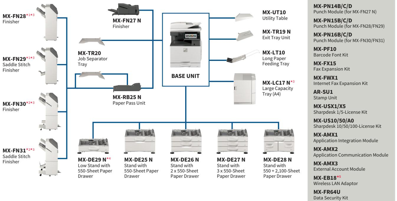
\*1: Max. paper capacity: 1,250 sheets \*2: Max. paper capacity: 3,250 sheets \*3: Requires MX-DE25 N/DE26 N/DE27 N/DE28 N. \*4: Cannot be used with MX-FN28/FN29/FN30/FN31/LC17 N. \*5: In some countries/regions, wireless LAN is standard-equipped (not optional) on the base unit.
