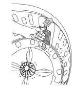
3. Attach lint filter box on washing tub to a downward direction.
