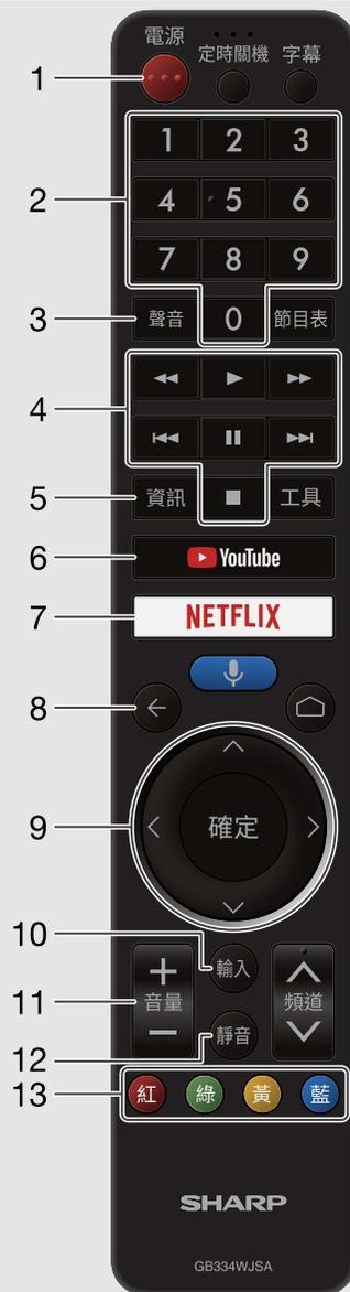
1 (電源) (POWER): Switch the TV power on or enter standby.
